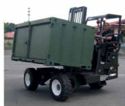
MOFFETT M8 - 4 Way in "Cat C" compliant version drives in forward, rearward, left and right direction
