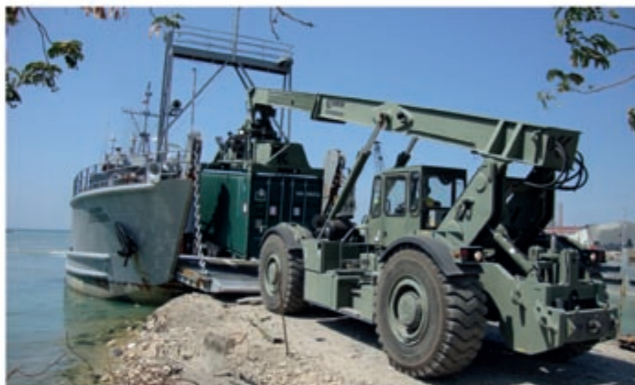
KALMAR RT240 RTCH unloading landing vessel
